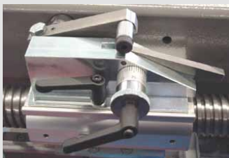
Il. 12: Mechanizm unoszenia sita. Pic. 12: Peel off device.
