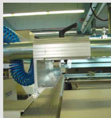
Il. 6: Regulowane szyny nośne sita. Pic. 6: Adjustable screen reception rails.
