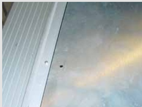
Il. 14: Kołki do mocowania ramy do folii. Pic. 14: Pins for fixing the foil frame.
