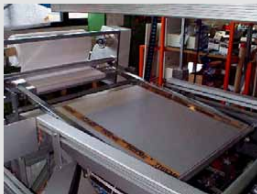
Il. 19: Mechanizm CleanPrint (stół drukarski). Pic.19: CleanPrint ink removal system (printing table).
