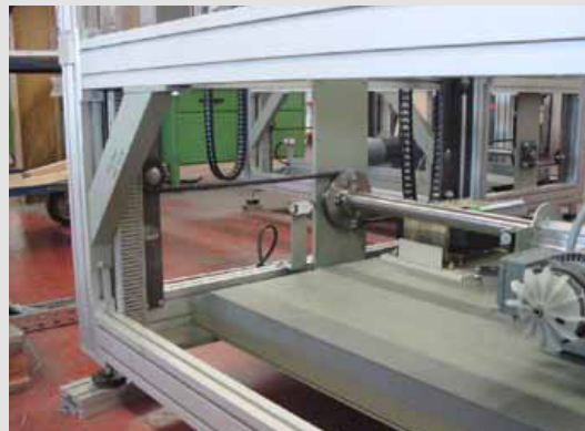
Il. 3: Anodowane elementy ramy. Pic. 3: Anodized parts of the chassis (covers removed).
