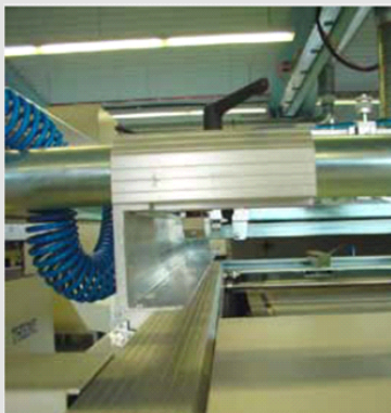
Il. 4: Regulowane szyny nośne sita. Pic. 4: Adjustable screen support bars.
