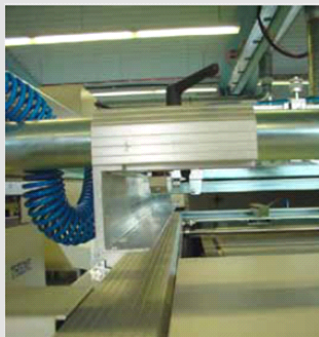
Il. 5: Regulowane szyny nośne sita. Pic.5: Adjustable screen support bars.
