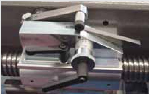
Il. 8: Mechanizm unoszenia sita. Pic. 8: Peel off device.
