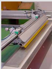
Il. 4: Opcjonalny mechanizm obracania rakla o 90°. Pic. 4: The optional 90° turn mechanism of the entire squeegee.
