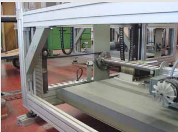
Il. 2: Anodowane elementy ramy. Pic. 2: Anodized parts of the chassis (covers removed).
