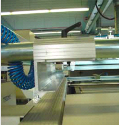
Il. 9: Regulowane szyny nośne sita. Pic.9: Adjustable screen reception rails.
