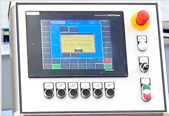
Il. 11: Panel sterowania THIEME GOT 1000. Pic. 11: THIEME Operation panel GOT 1000.
