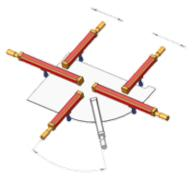
Freely programmable registration via servo axes For positioning of asymmetrical and symmetrical glass, the programmable axes allow for flexible positioning of the glass anywhere within registration station, with different aligning methods.
